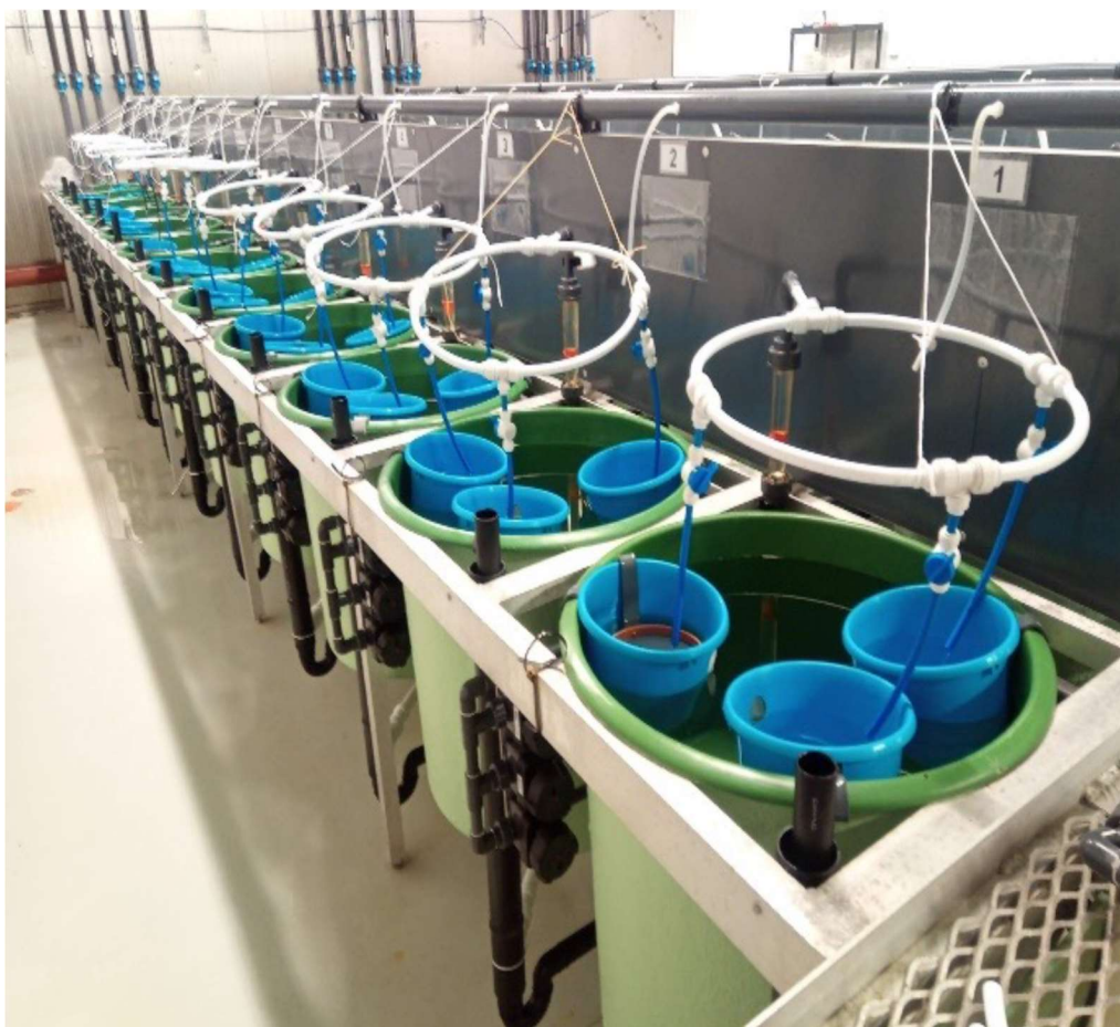
Figure 19. Setup of the incubation. From each tank/group four females were used for sampling for egg quality. Three sub-samples (triplicates) from each female were incubated as shown in the pictures. In triplicates, sampling for gene expression was done at unfertilized eggs (UE), early gastrula (EG) and newly hatched larvae (NHL).
